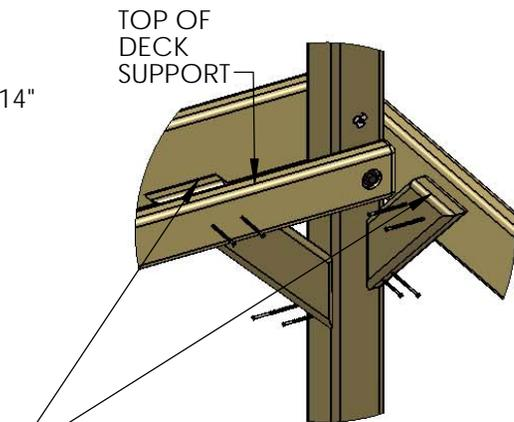
**\*\*IMPORTANT\*\*** - TOP OF ANGLE SUPPORT MUST BE FLUSH OR BELOW THE TOP OF THE DECK SUPPORT OR IT WILL INTERFERE WITH THE INSTALLATION OF THE DECK BOARDS.
