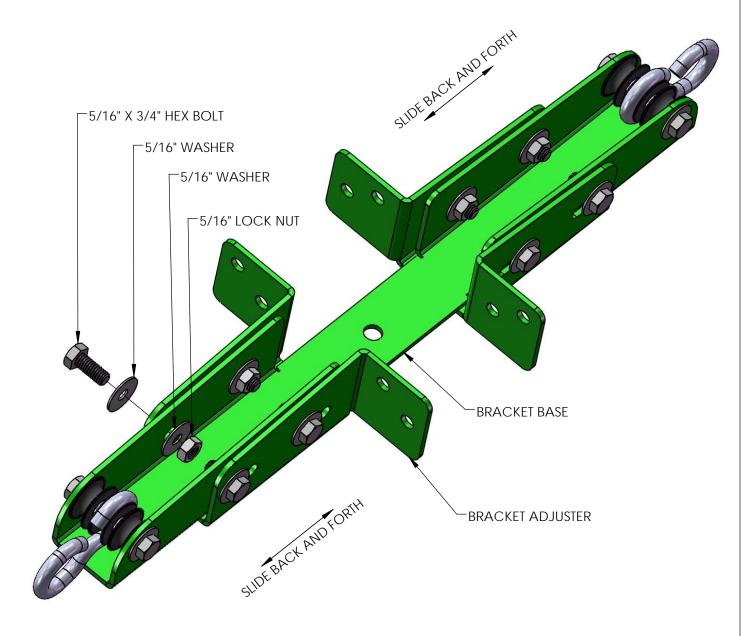
NOTE: DO NOT TIGHTEN BOLTS AND NUTS.
