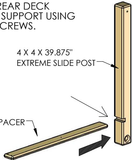
5: SECURE THE EXTREME SLIDE POST TO THE UPPER LEVEL UNDER DECK SUPPORT WITH A 3/8" X 5" LAG SCREW AND 3/8" WASHER THROUGH THE COUNTER SUNK HOLE.
