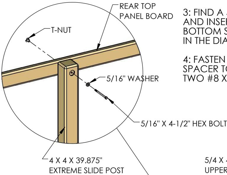
3: FIND A 5/4 X 4 X 36.75" UPPER REAR DECK SPACER AND INSERT IT INTO THE SLOT LOCATED AT THE BOTTOM SIDE OF THE EXTREME SLIDE POST AS SHOWN IN THE DIAGRAM BELOW.
