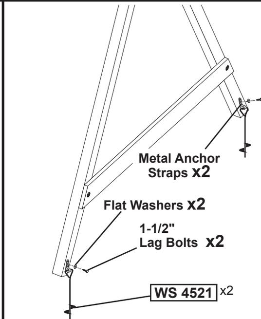
Install stakes into 3 x 3" uprights. Locate stakes as shown.
