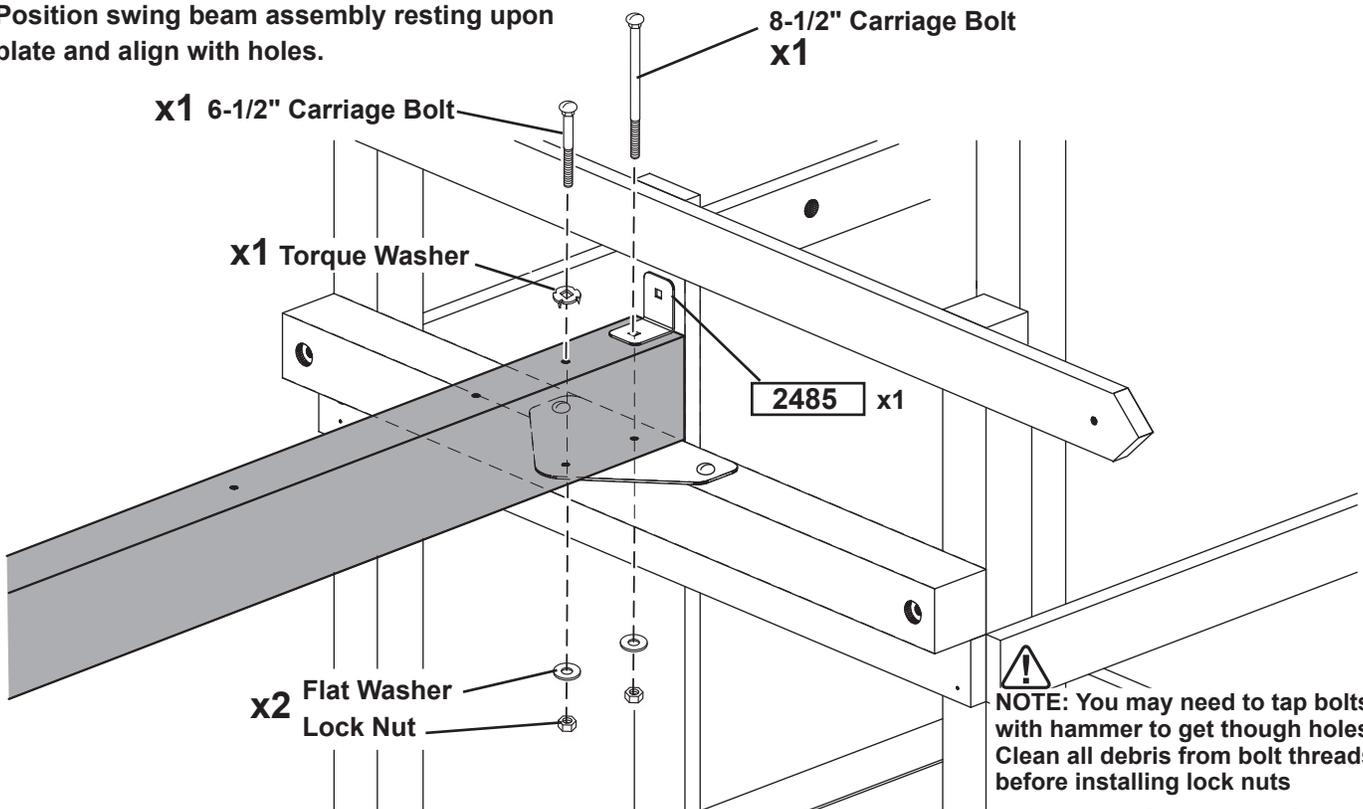
**NOTE:** You may need to tap bolts with hammer to get though holes. Clean all debris from bolt threads before installing lock nuts
