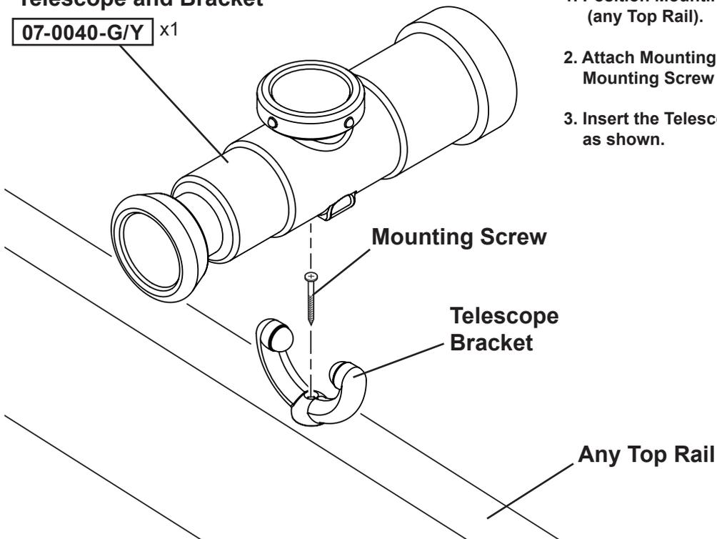
1. Position Mounting Bracket in desired location (any Top Rail).
