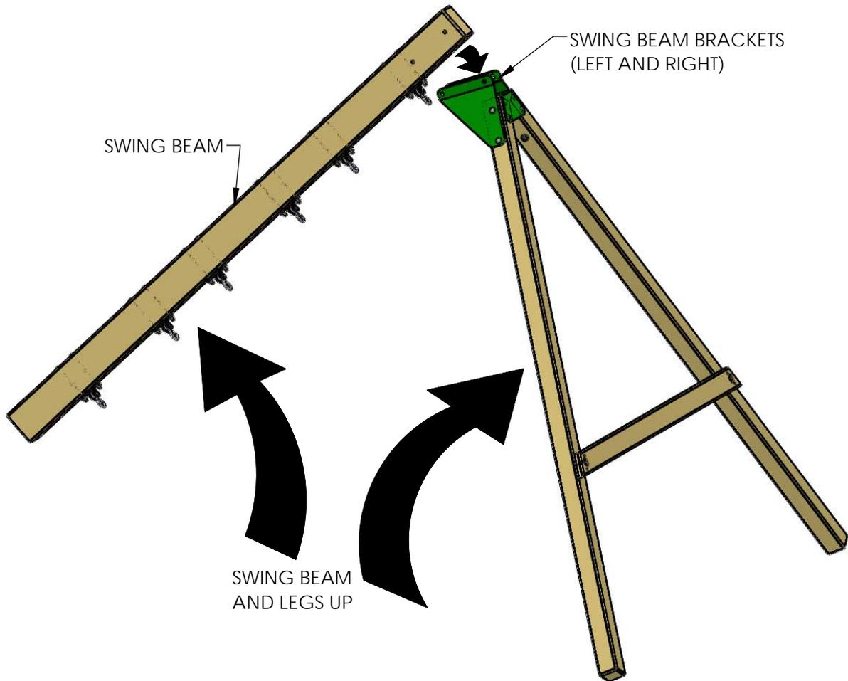
2: ASSEMBLE WITH FASTENERS AS SHOWN
