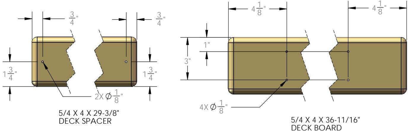
2: PLACE THE 5/4 X 4 X 29-3/8" DECK SPACERS BETWEEN THE CORNER POSTS. MAKE EACH DECK SPACER FLUSH TO THE INSIDE SURFACE OF THE 2 X 6 OR THE OUTSIDE SURFACE OF THE CORNER POSTS. DO NOT ATTACH THE DECK SPACERS YET.
