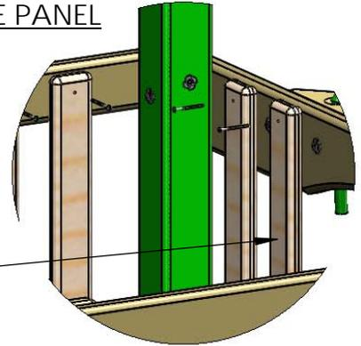
LEAVE THIS SLAT OFF UNTIL AFTER INSTALLING THE TIRE SWING BEAM. ONCE THE TIRE SWING BEAM IS IN PLACE SECURE THIS SLAT FLUSH TO THE SIDE OF THE SWING BEAM.
