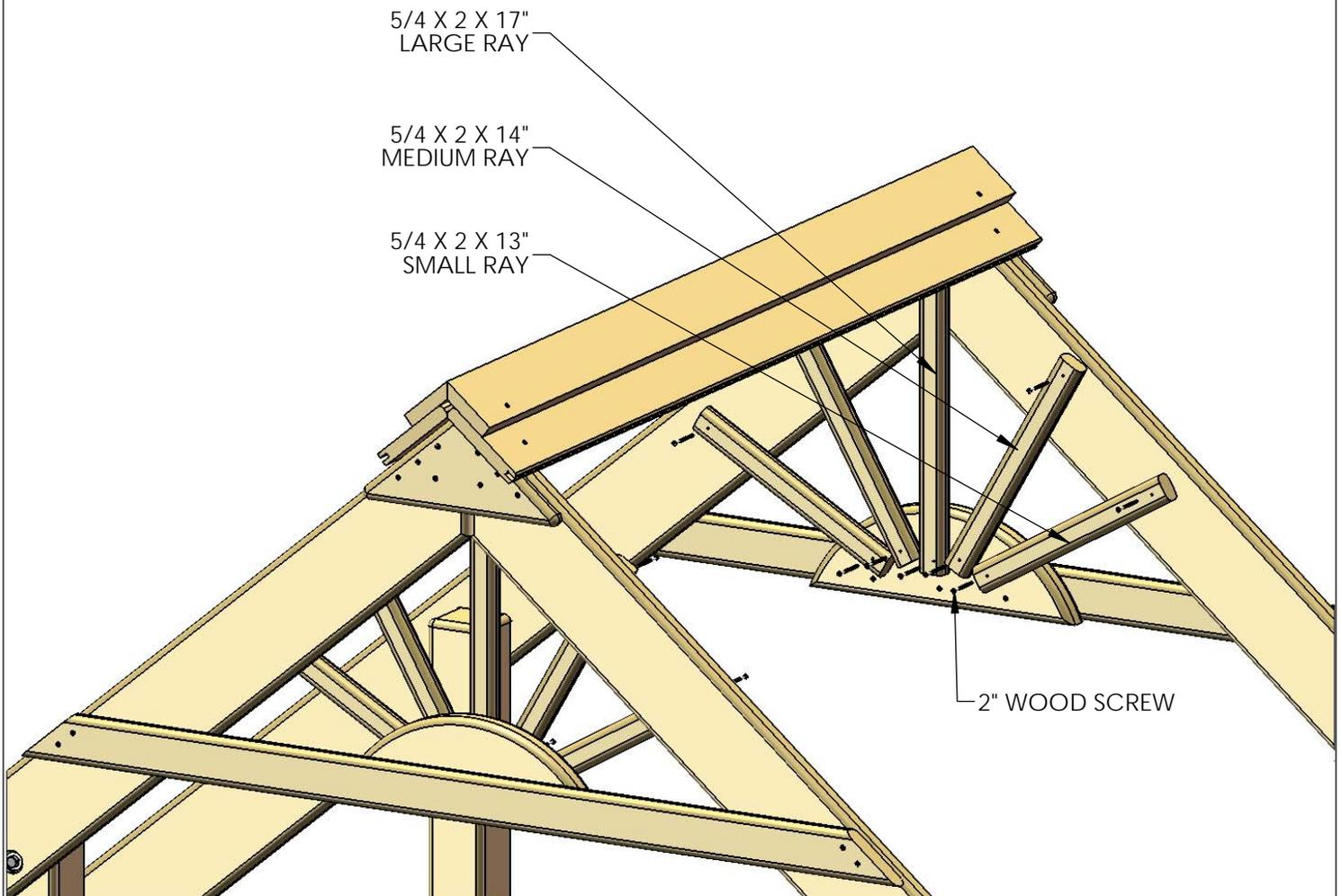
NOTE: ROOF BOARDS AND OTHER DETAILS OMITTED FOR CLARITY.
