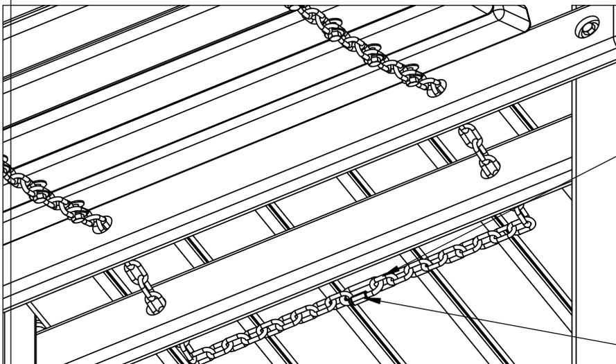
NOTE: TO ACHIEVE THE CORRECT GAP YOU MAY NOT BE CONNECTING THE END LINK OF EACH CHAIN. FOR EXAMPLE YOU MAY HAVE TO CONNECT THE SECOND, THIRD OR FORTH LINKS TOGETHER.
