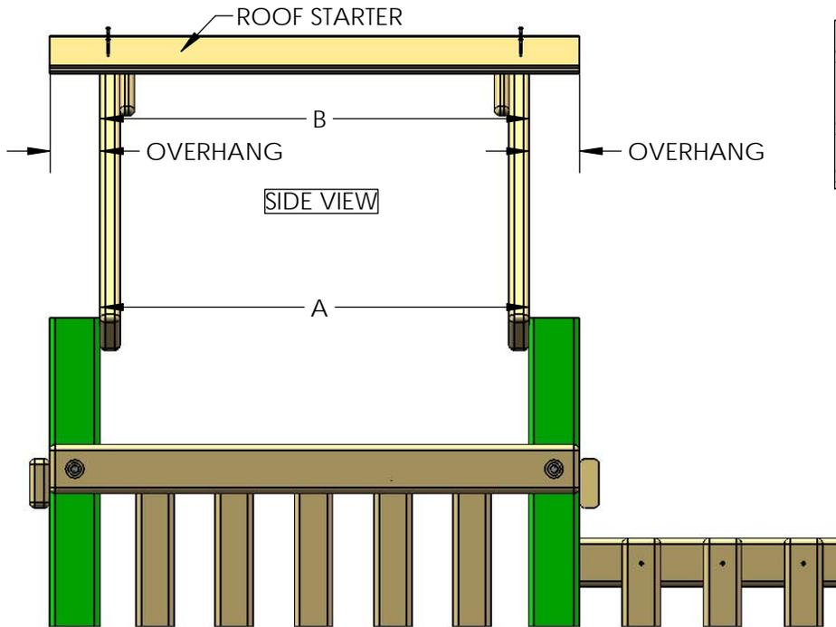
BEFORE INSTALLING THE ROOF STARTERS MAKE SURE DIMENSIONS A AND B MATCH. ALSO MAINTAIN THE SAME OVERHANG OF THE ROOF STARTERS ON EACH SIDE OF THE ROOF SUPPORTS.
