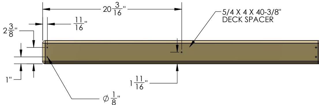
2: PLACE THE 5/4 X 4 X 40-3/8" DECK SPACER AT ONE END OF THE FORT. CENTER THE BOARD BETWEEN THE CORNER POSTS AND ATTACH IT WITH 2" WOOD SCREWS THROUGH THE PREDRILLED HOLES INTO THE DECK SUPPORT BELOW. NOTE THE TOP OF THE SCREW HEAD SHOULD BE FLUSH TO THE TOP OF THE DECK SPACER.
