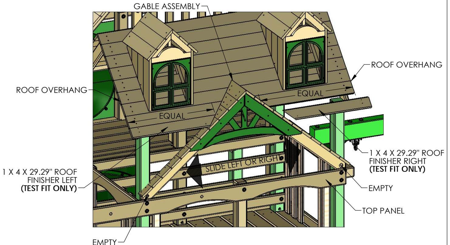
3: AFTER THE GABLE ASSEMBLY IS IN ITS FINAL POSITION. GO INSIDE ON TOP OF THE DECK AND PULL THE GABLE ASSEMBLY TOWARDS YOU MAKING SURE IT IS FLUSH TO THE OUTSIDE OF THE ROOF AND INSERT TWO 1-1/2" WOOD SCREW FROM UNDERNEATH THE ROOF INTO THE GABLE ASSEMBLY ROOF PEAK. USE THE DIMENSIONS SHOWN IN THE DIAGRAM TO THE LEFT TO INSERT THE WOOD SCREWS IN THE CORRECT LOCATION. **REMOVE THE ROOF FINISHERS, THESE WILL BE USED IN A LATER STEP.**
