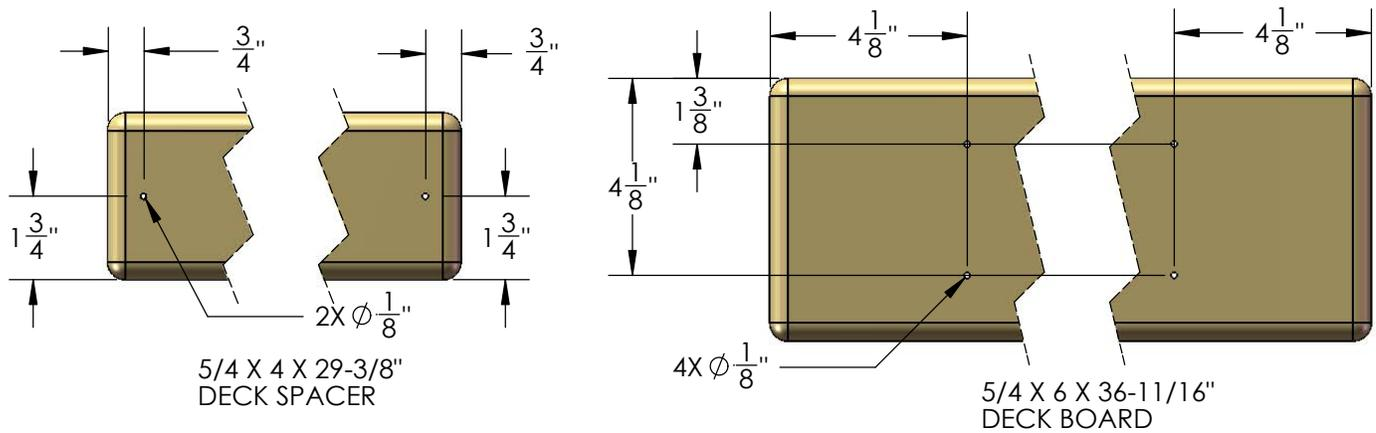
2: PLACE THE 5/4 X 4 X 29-3/8" DECK SPACERS BETWEEN THE CORNER POSTS. MAKE EACH DECK SPACER FLUSH TO THE INSIDE SURFACE OF THE 2 X 6. ATTACH EACH DECK SPACER TO THE DECK SUPPORTS WITH TWO 2" WOOD SCREWS. NOTE THE TOP OF THE SCREW HEAD SHOULD BE FLUSH WITH THE TOP OF THE DECK SPACER.
