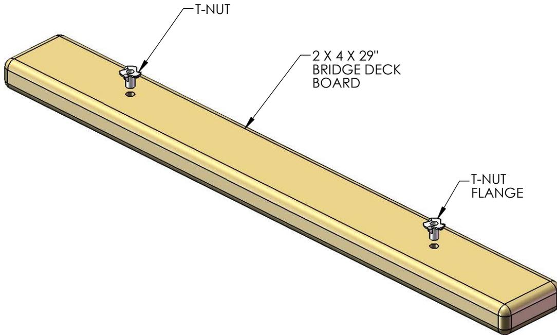
2: FLIP ALL 15 BRIDGE DECK BOARDS OVER SO THAT THE FLANGE OF THE T-NUT IS FACING DOWN. LAY THE BRIDGE DECK BOARDS OUT ON A FLAT SURFACE AS SHOWN BELOW.
