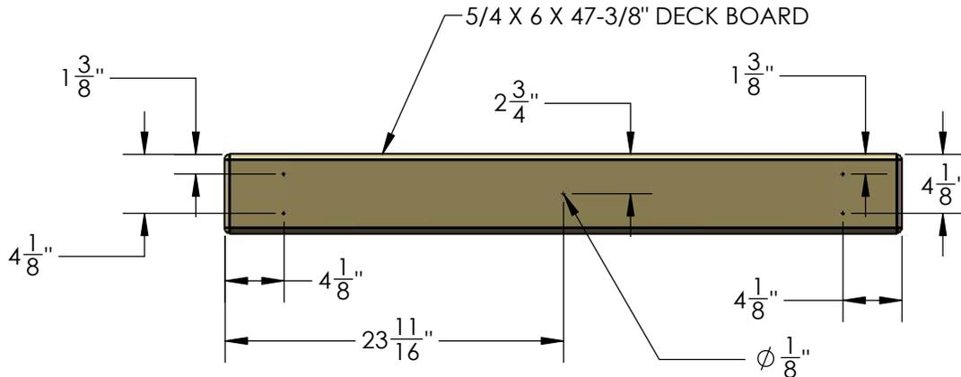
2: START WITH A 5/4 X 6 X 47-3/8" DECK BOARD AT ONE END OF THE FORT. CENTER THE BOARD BETWEEN THE FRONT FACE BOARD AND THE REAR BOTTOM PANEL BOARD AND ATTACH IT WITH 2" WOOD SCREWS THROUGH THE PREDRILLED HOLES AND INTO THE DECK SUPPORTS BELOW. LEAVE A UNIFORM (APPROX. 1/4") SPACE BETWEEN THE DECK BOARDS. NOTE: THE TOP OF THE SCREW HEAD SHOULD BE FLUSH TO THE TOP OF THE DECK BOARDS.
