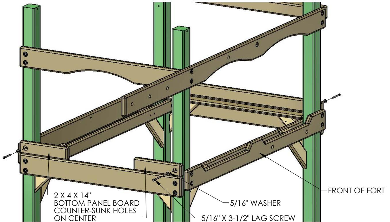
2: PLACE THE 2 X 4 X 47-1/2" BOTTOM PANEL BOARD ON TOP OF THE 2 X 6 PANEL BOARD WITH OFFSET HOLES UP AND FASTEN TO THE CORNER POSTS WITH 5/16" X 3-1/2" LAG SCREWS AND 5/16" WASHERS.
