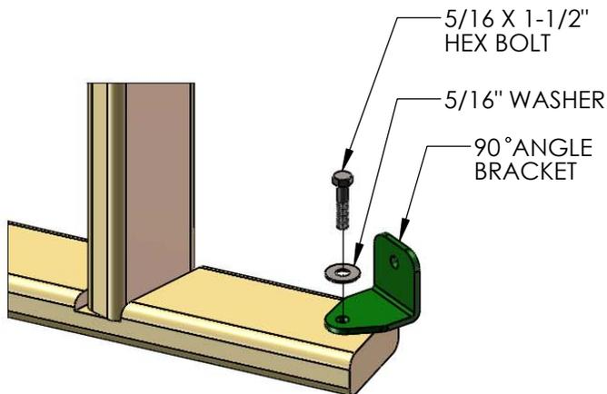
7: INSTALL THE 90° ANGLE BRACKETS TO THE INSIDE OF THE LADDER RAILS WITH 5/16 X 1-1/2" BOLTS, 5/16 WASHERS, INTO THE 5/16" T-NUTS.
