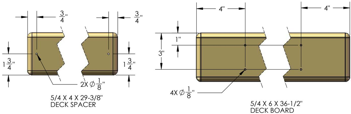
2: PLACE THE 5/4 X 4 X 29-3/8" DECK SPACERS BETWEEN THE CORNER POSTS. MAKE EACH DECK SPACER FLUSH TO THE INSIDE SURFACE OF THE 2 X 6. ATTACH EACH DECK SPACER TO THE DECK SUPPORTS WITH TWO 2" WOOD SCREWS. NOTE THE TOP OF THE SCREW HEAD SHOULD BE FLUSH WITH THE TOP OF THE DECK SPACER.
