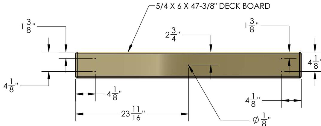
2: START WITH A 5/4 X 6 X 47-3/8" DECK BOARD AT ONE END OF THE FORT. CENTER THE BOARD BETWEEN THE FRONT FACE BOARD AND THE REAR BOTTOM PANEL BOARD AND ATTACH IT WITH 2" WOOD SCREWS THROUGH THE PREDRILED HOLES AND INTO THE DECK SUPPORTS BELOW. LEAVE A UNIFORM (APPROX. 1/4") SPACE BETWEEN THE DECK BOARDS. NOTE: THE TOP OF THE SCREW HEAD SHOULD BE FLUSH TO THE TOP OF THE DECK BOARDS.
