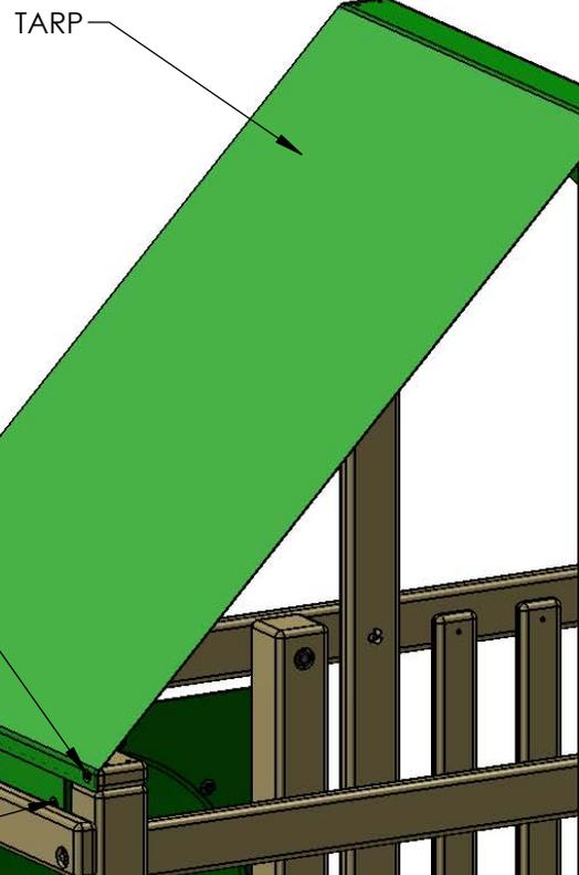
FASTEN OUTSIDE GROMMETS FIRST TO THE SIDE OF THE TARP BOARD ON EACH SIDE WITH #14 X 1-1/4" PAN HEAD SCREWS AND 1/4" WASHERS. REPEAT FOR OTHER SIDE.
