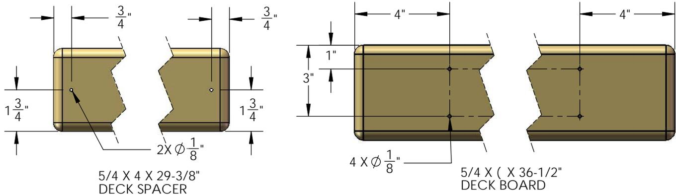
2: PLACE THE 5/4 X 4 X 29-3/8" DECK SPACERS BETWEEN THE CORNER POSTS. MAKE EACH DECK SPACER FLUSH TO THE INSIDE SURFACE OF THE 2 X 6. ATTACH EACH DECK SPACER TO THE DECK SUPPORTS WITH TWO 2" WOOD SCREWS. NOTE THE TOP OF THE SCREW HEAD SHOULD BE FLUSH WITH THE TOP OF THE DECK SPACER.
