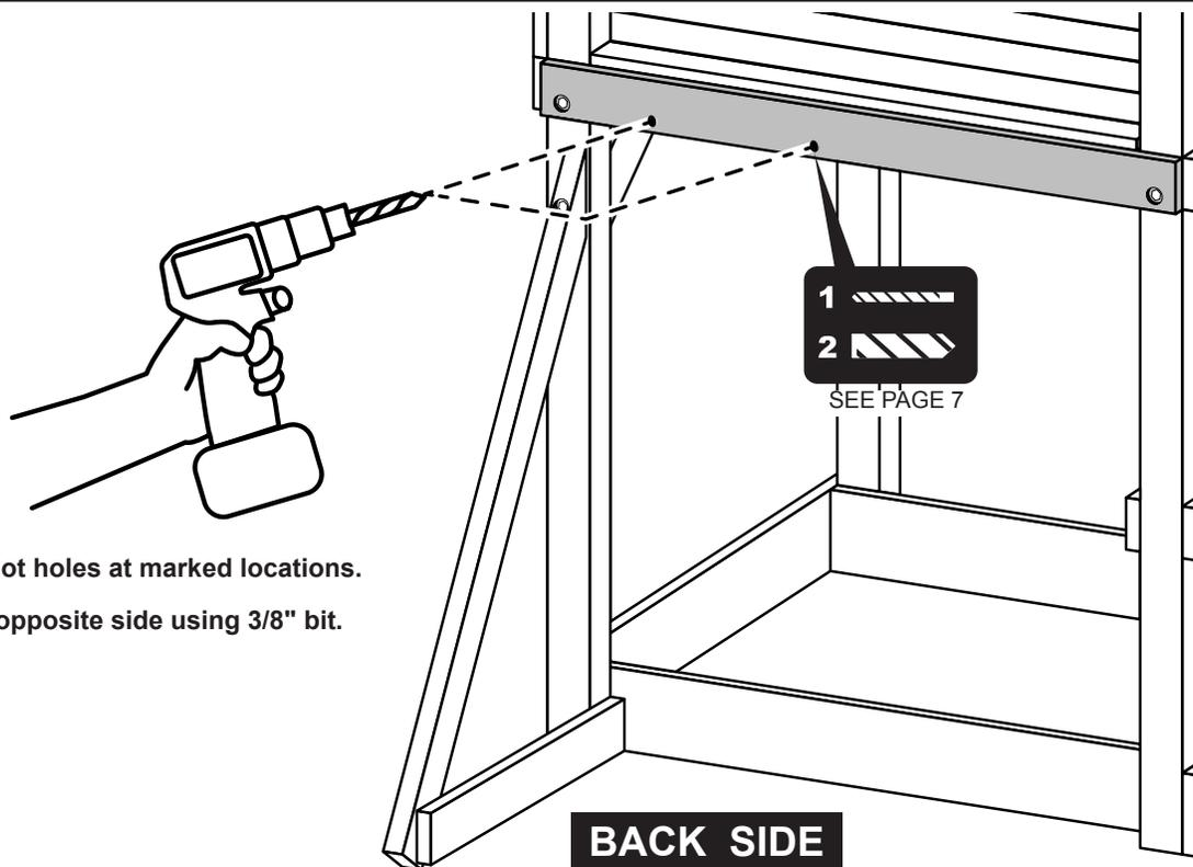
Pre-drill two 1/4" pilot holes at marked locations.
