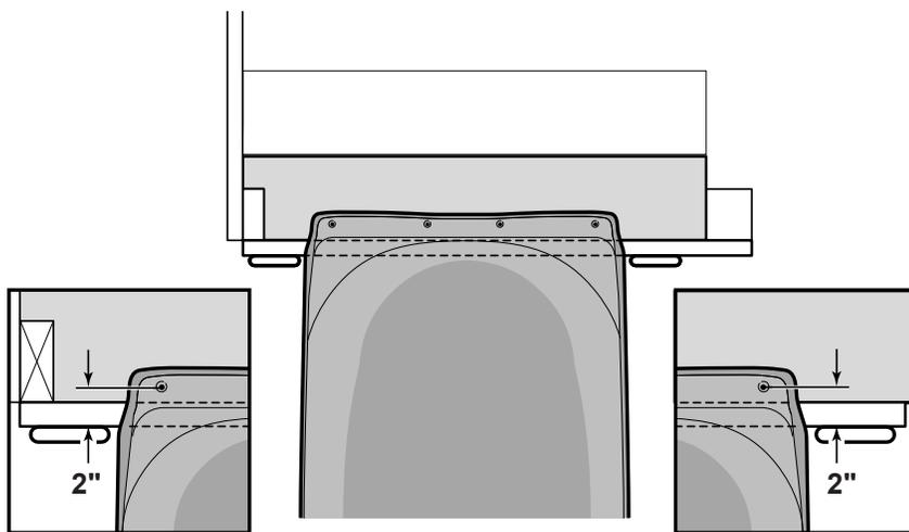
Measure and locate holes 2" from edge of deck.
