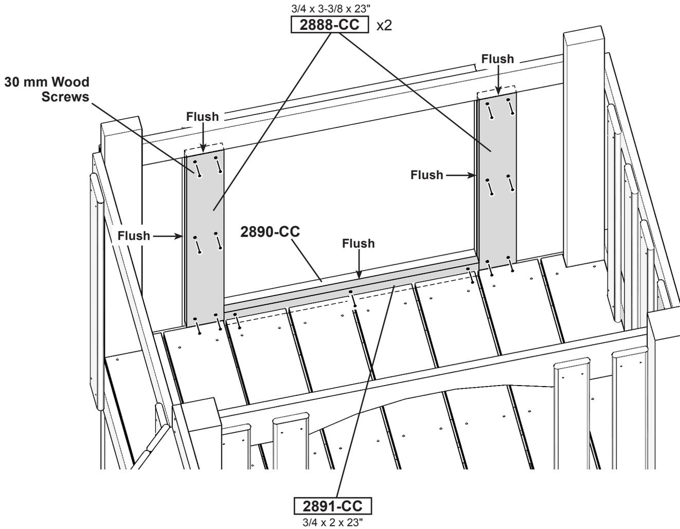
Insert 2891-CC between deck boards and 2890-CC.
