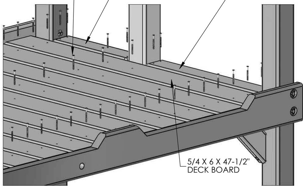
2: START WITH A 5/4 X 6 X 47-3/8" DECK BOARD AT ONE END OF THE FORT. CENTER THE BOARD BETWEEN THE FRONT FACE BOARD AND THE REAR BOTTOM PANEL BOARD AND ATTACH IT WITH 2" WOOD SCREWS THROUGH THE PREDRILED HOLES AND INTO THE DECK SUPPORT BELOW. LEAVE A UNIFORM (APPROX. 1/4") SPACE BETWEEN THE DECK BOARDS. NOTE: THE TOP OF THE SCREW HEAD SHOULD BE FLUSH TO THE TOP OF THE DECK BOARDS.
