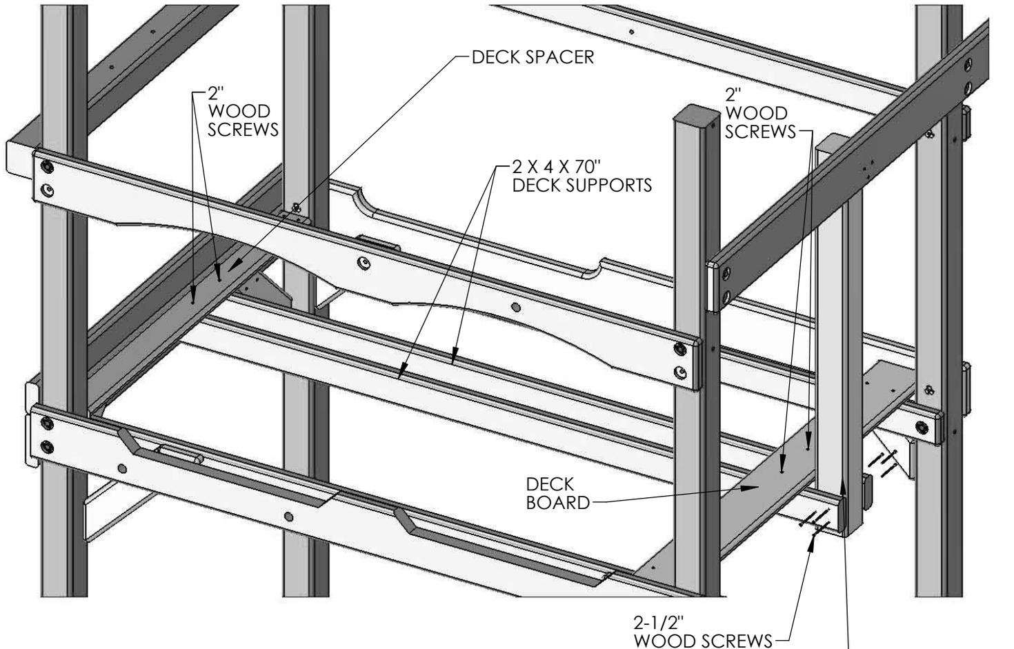
HAVE AN ASSISTANT HOLD THE END OF THE DECK SUPPORTS WHILE YOU PUT IN SCREWS THROUGH DECK BOARD AND DECK SPACER.
