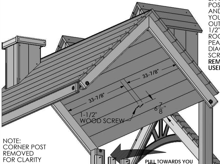
3: AFTER THE GABLE ASSEMBLY IS IN ITS FINAL POSITION. GO INSIDE ON TOP OF THE DECK AND PULL THE GABLE ASSEMBLY TOWARDS YOU MAKING SURE IT IS FLUSH TO THE OUTSIDE OF THE ROOF AND INSERT TWO 1-1/2" WOOD SCREWS FROM UNDERNEATH THE ROOF INTO THE GABLE ASSEMBLY ROOF PEAK. USE THE DIMENSIONS SHOWN IN THE DIAGRAM TO THE LEFT TO INSERT THE WOOD SCREWS IN THE CORRECT LOCATION. REMOVE THE ROOF FINISHERS, THESE WILL BE USED IN A LATER STEP.
