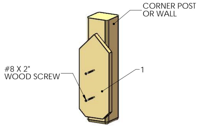
ATTACH THE WALL 1 TO THE CORNER POST OR WALL WITH #8 X 2" WOOD SCREW.
